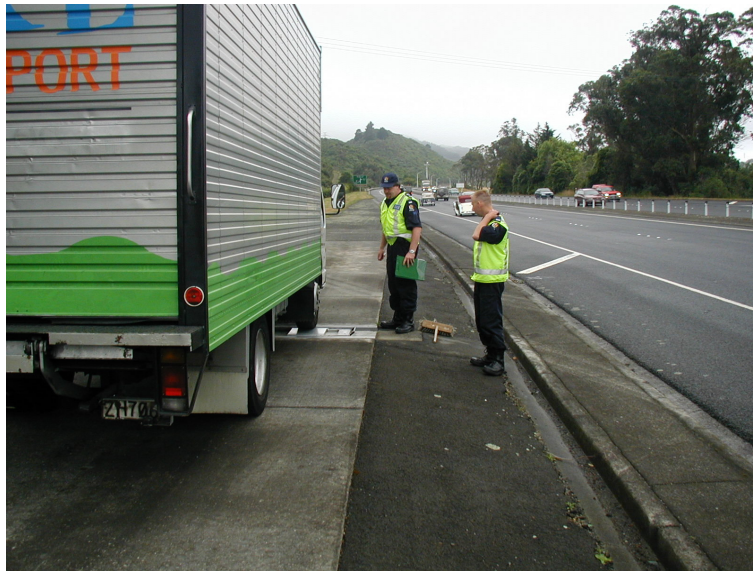
Photo 5.3 Weigh Pits State Highway 2, Haywards, Wellington.
