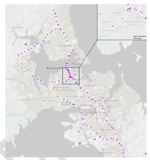
AT has a limited number of cameras being used with a VMS based ANPR solution to enforce special use lane compliance (bus only lanes). It is also used for measuring journey times by recording the time for unique vehicles to travel between fixed locations.
