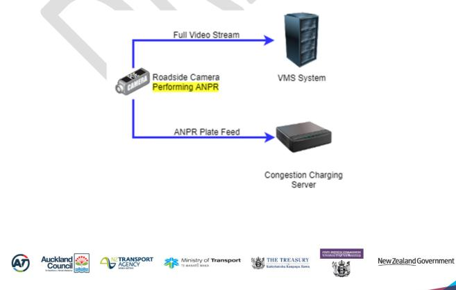
FIGURE 15: NEW CAMERAS - CAMERA PERFORMS ANPR AND VMS ALSO RECEIVES VIDEO FEED
