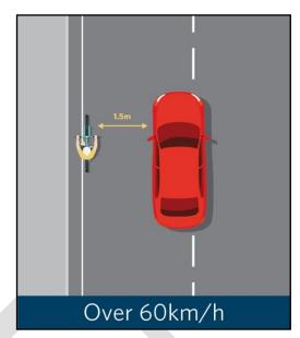
Figure 5A: The minimum overtaking gap for motor vehicles passing cycles, transport devices, horses, pedestrians and people using mobility devices will be 1m when the speed limit is 60km/h or less, or 1.5m when the speed limit is above 60km/h. Drivers must be safe and considerate when driving past road users in different lanes (such as cycle lanes).
