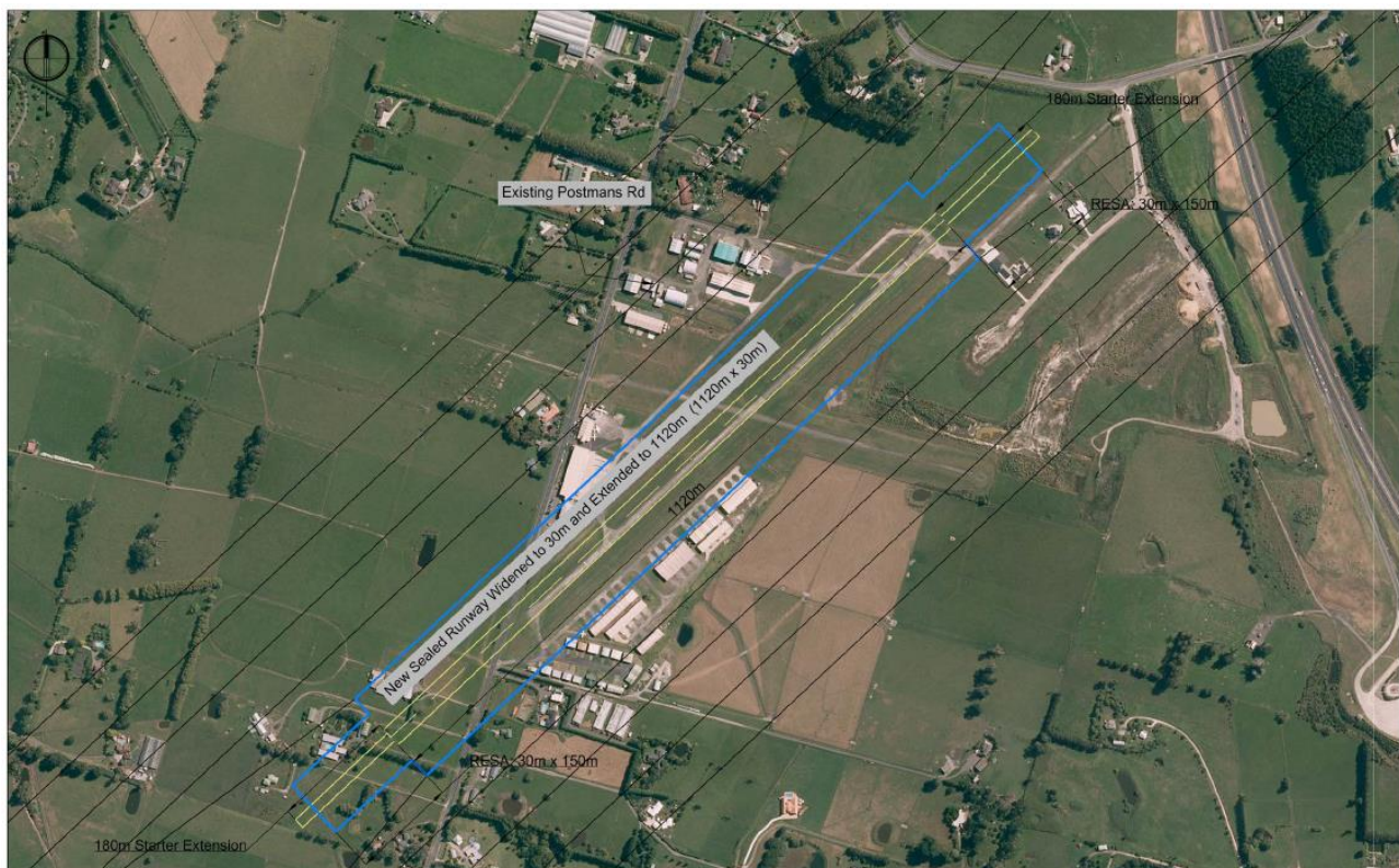
Figure 11: Stage 3 runway extension
